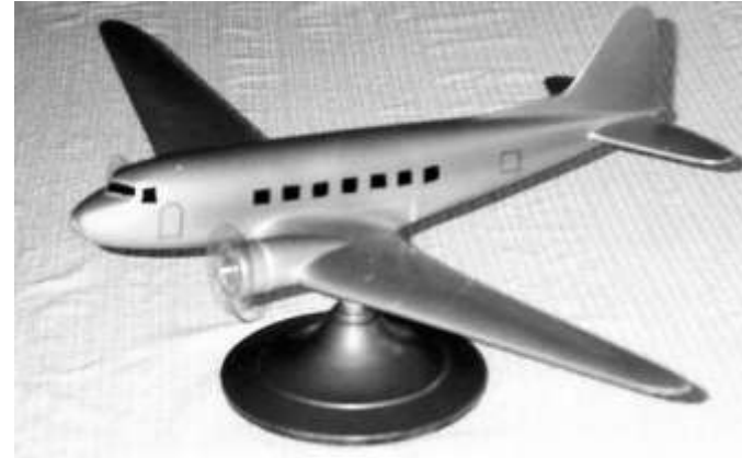
Ground Plane Tests Aluminum Coated Scale Model DC-3
