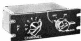
Control Panel C-245A/ARC-2
